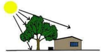
Figure 2. An air conditioning unit on a south or west wall should be protected from the sun.
